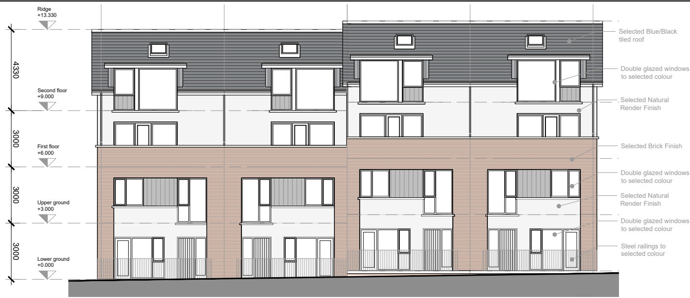
Front Elevation (Waterfall Road) - Scale 1:200
